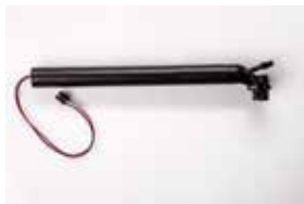
Invisible Performance Package electronics in the seat post
